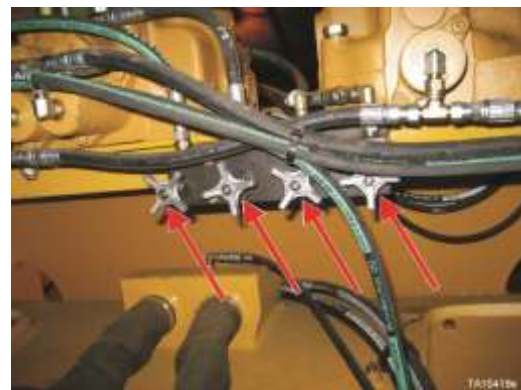
Pressure bleed down valves
