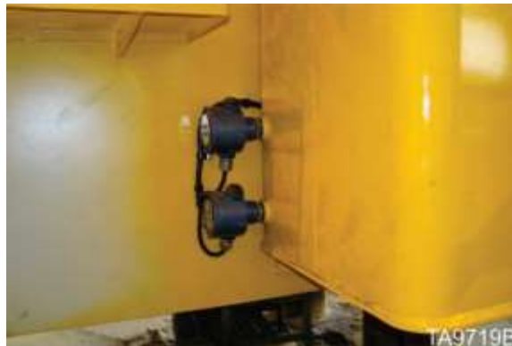
Figure 3. Hydraulic reservoir heaters (typical)
